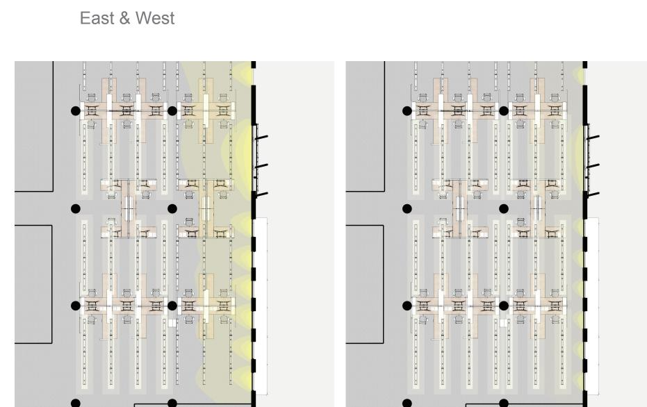
A smarter lighting design will help to provide even adequate lighting throughout the day, without over exposing those by the window or leaving others in the dark. Having lights running parallel to the exterior wall and set to different controls will allow for artificial lighting to be used by the window only when the sunlight in not sufficient.
