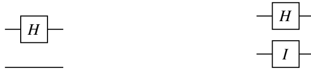
(a) A quantum gate acting on one out of two qubits. (b) Insertion of an identity gate.
