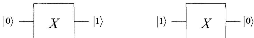
Figure 1.1: Inverter or the NOT quantum logic gate U . The wires carry quantum information, namely qubits.
