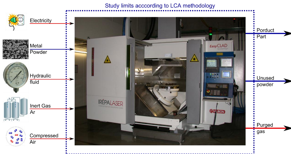
Figure 17. Directed energy deposition (CLAD) process.
