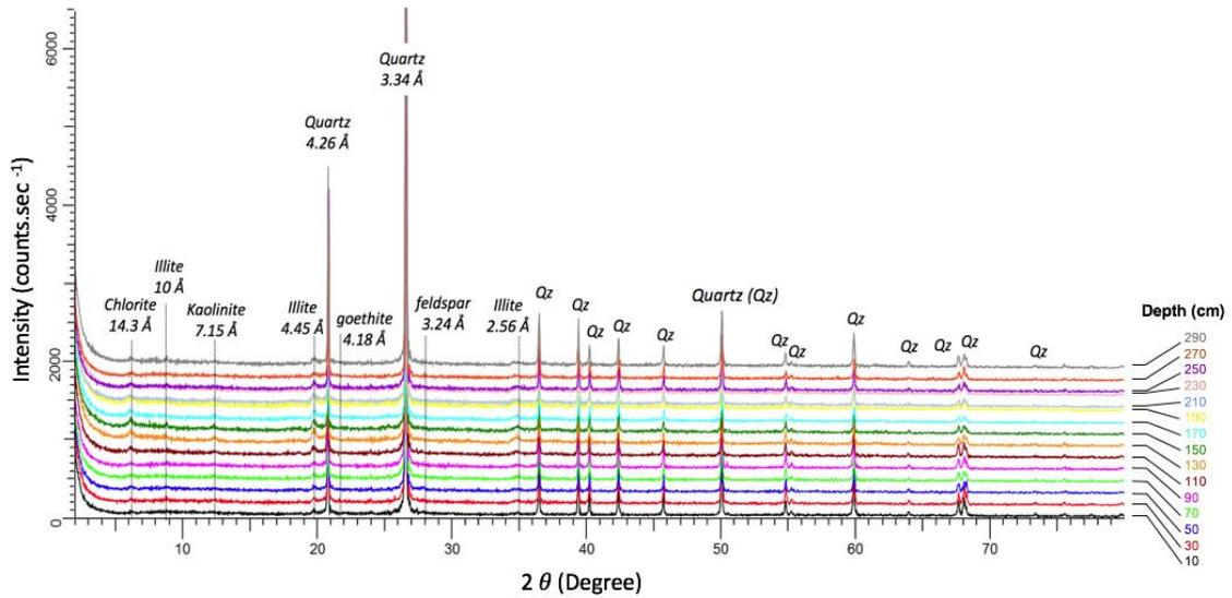
**Figure 4.6:** X-ray diffractograms (XRD) of the bulk soil samples collected every 20 cm along the 300-cm deep soil profile.
