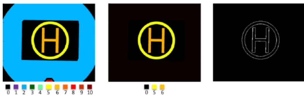
Figure 2.3: The left hand side indicates all the possible candidates identified before the cascade check, the middle is the final helipad marks represented by the two remaining blobs and the right hand side is the contours of helipad.
