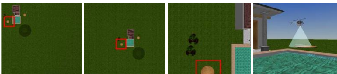
Figure 2.9: Starting from left to right, the leftmost is the initial frame when the vision algorithm detects the features, followed by the UAV reaches the target and it attempts to descend a little as well as the rightmost simulated 3D environment, respectively.
