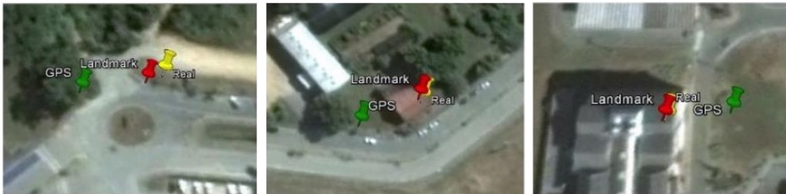
Figure 2.8: Auto-localization position comparison between GPS, landmark recognition estimation and real UAV position for the roundabout (left), roof of a house (middle) and roof (right), respectively.
