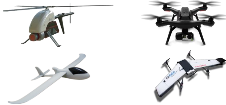
Figure 1.1: The top left is single rotor, top right is multi-rotor, bottom left is fixed-wing and the bottom right is hybrid UAV, respectively.
