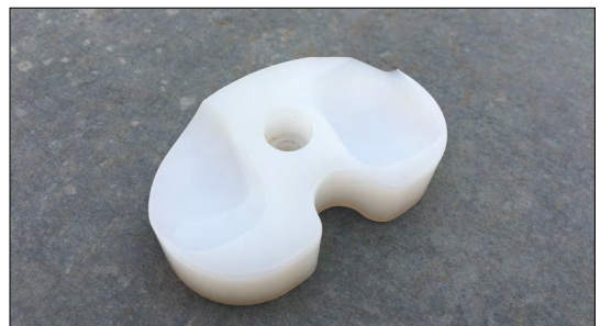
Figure 6. CNC milled tibial prosthesis geometry
