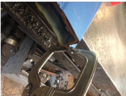
Figure 3. Cutting the samples from the B pillar for the analysis
