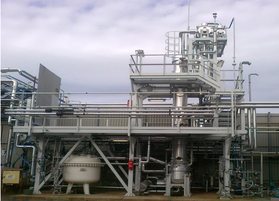
Figure 4: Industrial distillation column for treatment of process wastewater (Toth, 2015)
