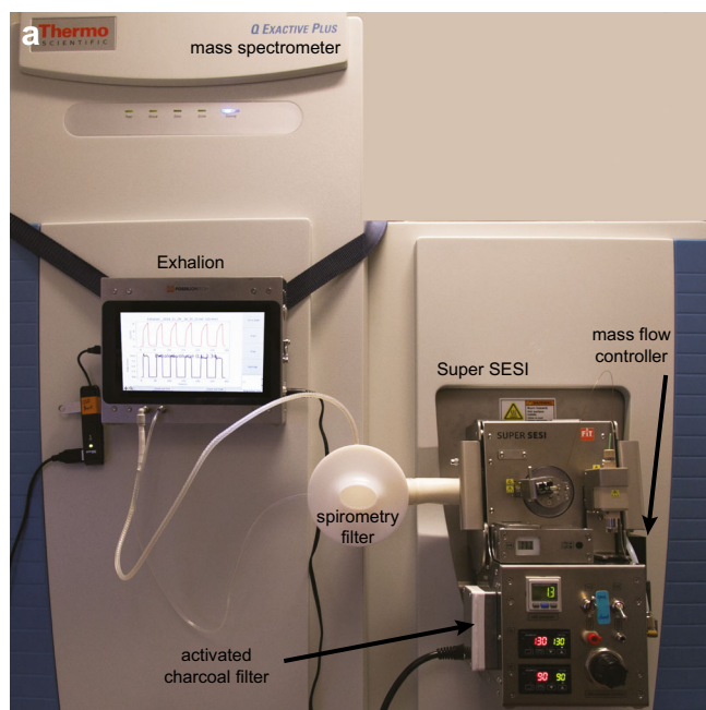
Fig. 1 Real-time breath analysis using SESI-HRMS. a SESI-HRMS analytical platform located in a clinical setting (University Children's Hospital Basel) dedicated for real-time breath analysis. The system features three main elements: (i) exhalation interface, which provides feedback to the participants on the exhalation maneuver; (ii) ion source, which efficiently ionizes exhaled metabolites, and (iii) high-resolution mass
