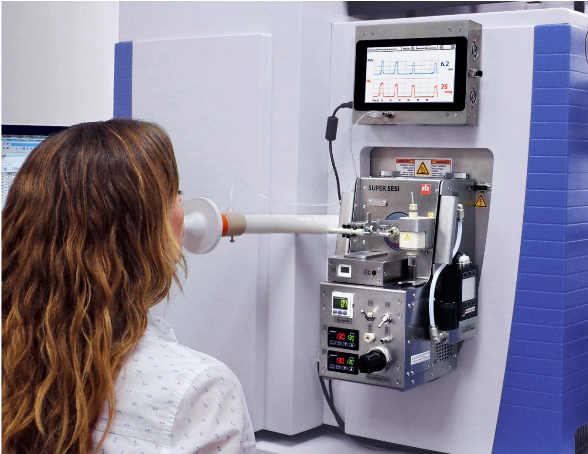
Fig. S2 A pictorial representation of a subject exhaling into the real-time breath analysis platform used in this study
