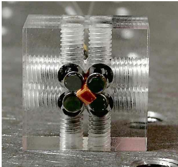
Figure 7.8: Photograph of the housing for four collimators.
