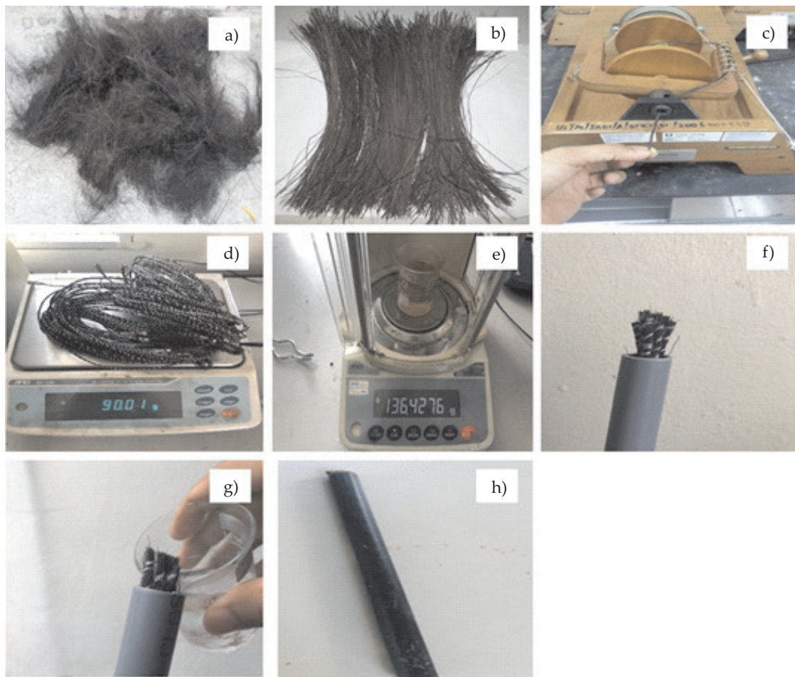
Fig. 2. Photograph of: a) raw sugar palm fiber, b) combed sugar palm fiber, c) spinning process [44, 49], d) sugar palm yarn fiber, e) weighed epoxy resin, f) inserted sugar palm yarn fiber into the PVC pipe, g) the pouring process, h) cured composite
