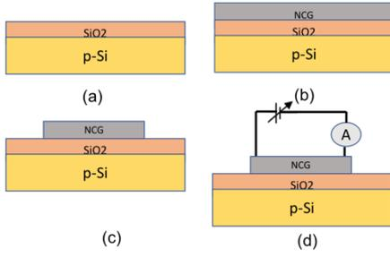
Fig.1. Device Fabrication Process (a) SiO<sub>2</sub> layer deposited on p-Si (b) NCG deposition (c) NCG patterning (d) Schematic of NCG/p-Si resistive device
