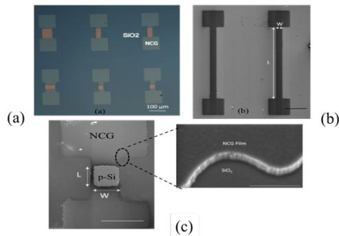
Fig. 3. (a) Optical microscope images of NCG devices with various dimensions, (b) Scanning electron microscope (SEM) image of NCG resistive strip on SiO<sub>2</sub>/p-Si layer. Scale bar is 100 μm, (c) SEM image of a single Schottky device structure. Scale bar is 50 μm, (inset) Enlarged view of NCG deposition on SiO<sub>2</sub> layer. Scale bar is 500 nm.
