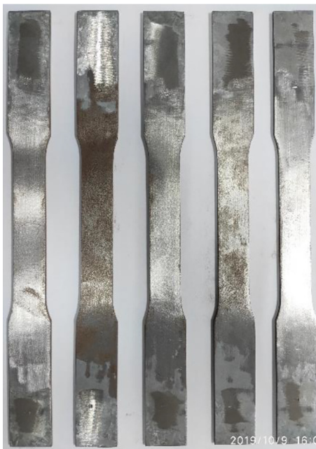
a) Coupon sample for CFS properties
