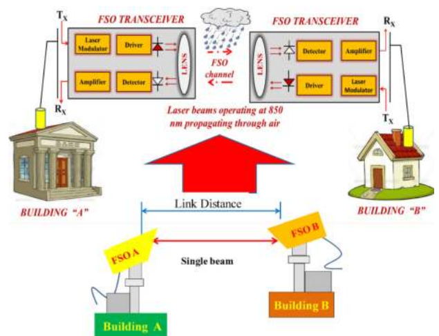
FIGURE 2. Overview of single beam FSO communication system in static placement [18].
