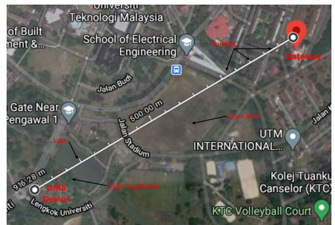
FIGURE 2. Location of the LoRa device and GW, University of Technology Malaysia, Johor Bahru.
