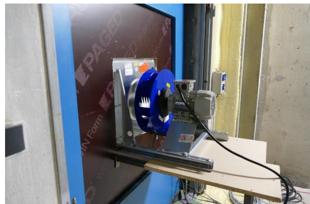
Figure 4: Top view layout of the test facility (left) and view of the outlet pressure chamber with the fan assembly (right)
