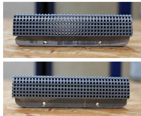
(h) Structured porosities with and without separating layer.
