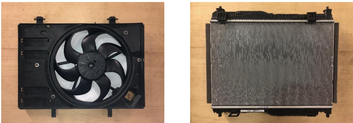
Figure 1: Automotive engine cooling module; left: fan system and shroud; right: heat exchanger.
