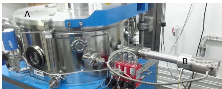
Figure 3.52: Homemade plasma oxygen source co-sputtering set up. A: Vacuum chamber for thin film deposition. B: Quartz tube for plasma generation
