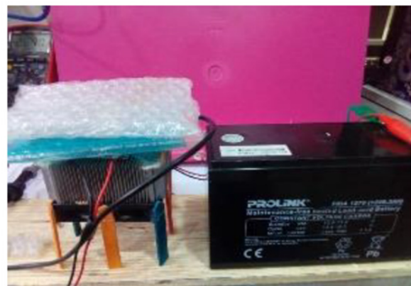
FIGURE 12. Power supply (12V) & thermoelectric module with heat sink
