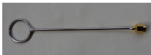
FIGURE 5. Handcrafted magnetic field probe Source: Neilhao (2013)
