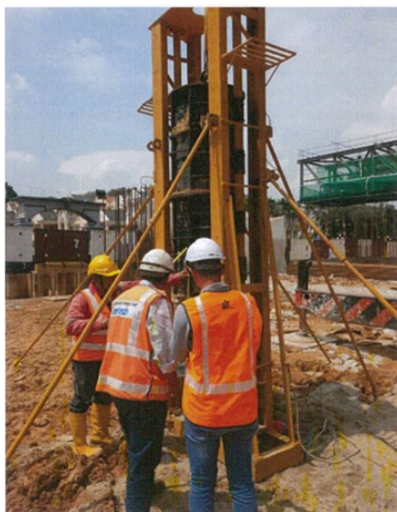
FIGURE 5. PDA setup for MC 23
