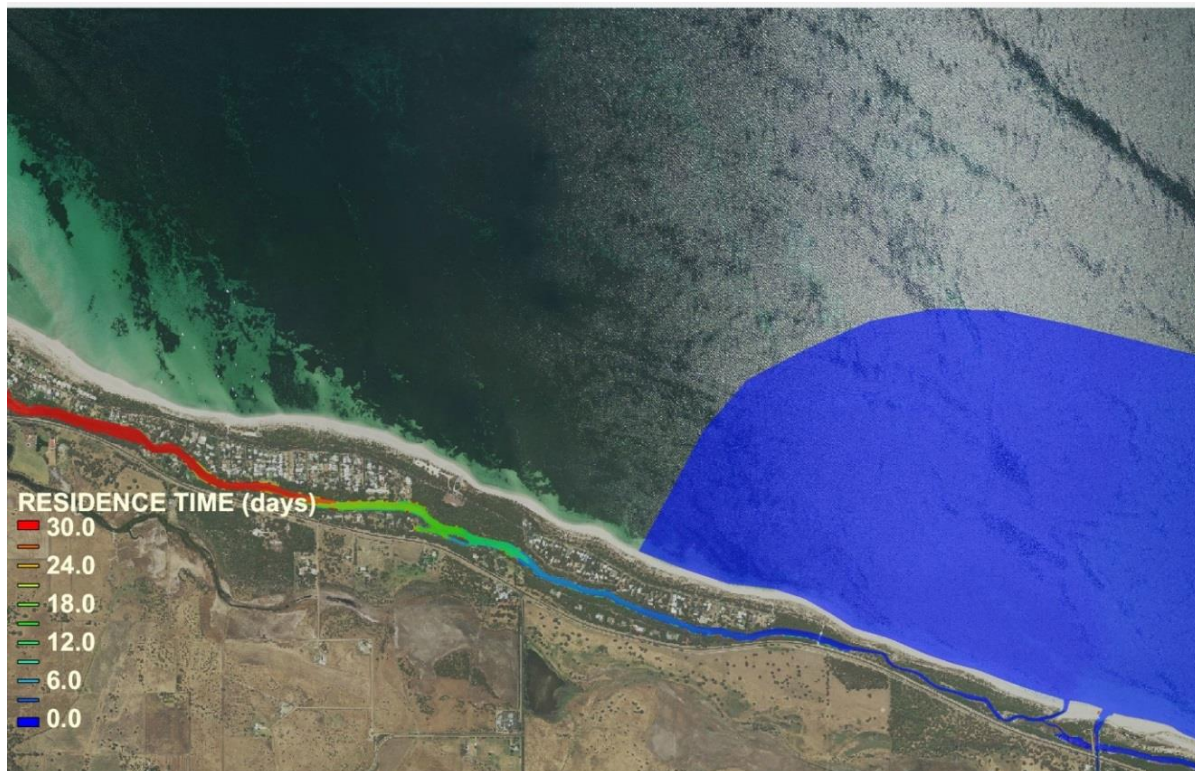
Fig. 13. Heat map showing the residence time ( i.e. the time required for a hypothetical tracer introduced into the system to be reduced to a third of its original concentration) for waters in Toby Inlet and the Deadwater under a scenario where, as occurred in March 2018, the bar at the mouth of Toby Inlet was open, but that of Station Gully was closed, with the culvert between the two systems open. Values obtained from advection-dispersion module built for Toby Inlet using TUFLOW-FV by the Department of Water and Environmental Regulation. Taken from Frazer and Hall (2018).
