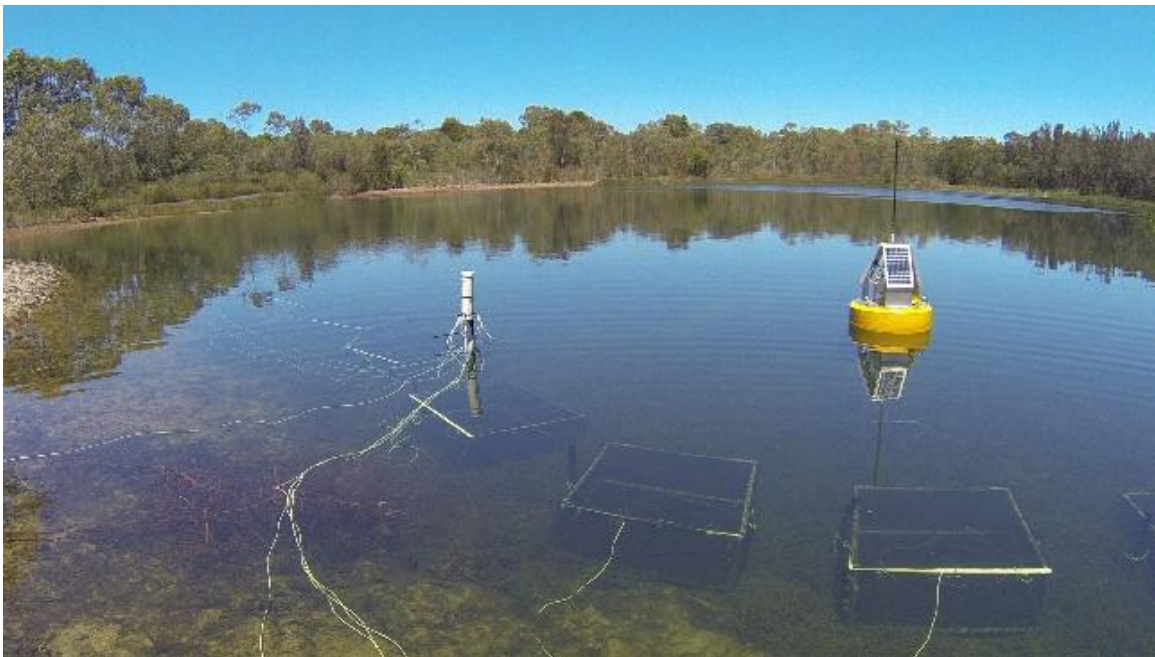
Figure 1: The relocation cages, valvometer and water quality monitoring loggers at Taylor's Lake in November 2019.
