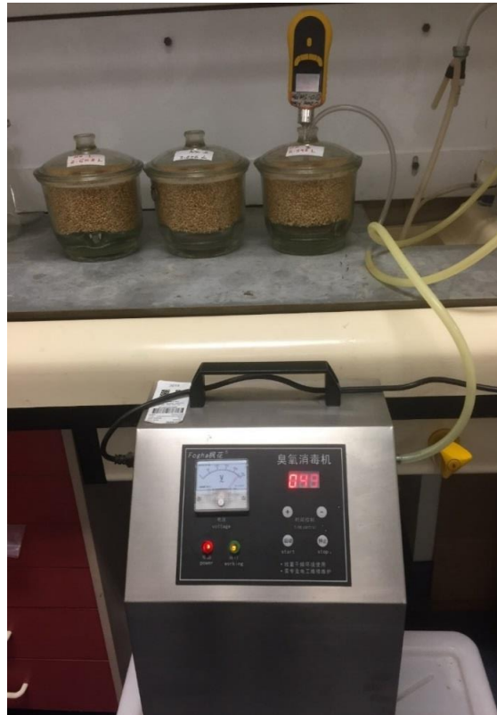
Figure 2.1. Fumigation procedures with ozone.
