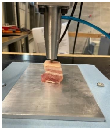
Figure 17. Close-up of porcine tissue and jet injector nozzle.
