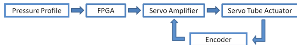
Figure 4. Block diagram of semi-closed-loop servo-tube injector.
