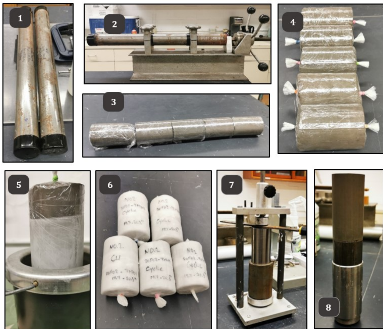
Figure 4.7: Marine clay samples' preparation: extraction from Shelby tubes, segmentation, wax-coating, and labeling.
