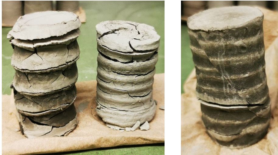
Figure 4.42: Marine clay samples after testing and air drying for 48 Hours.
