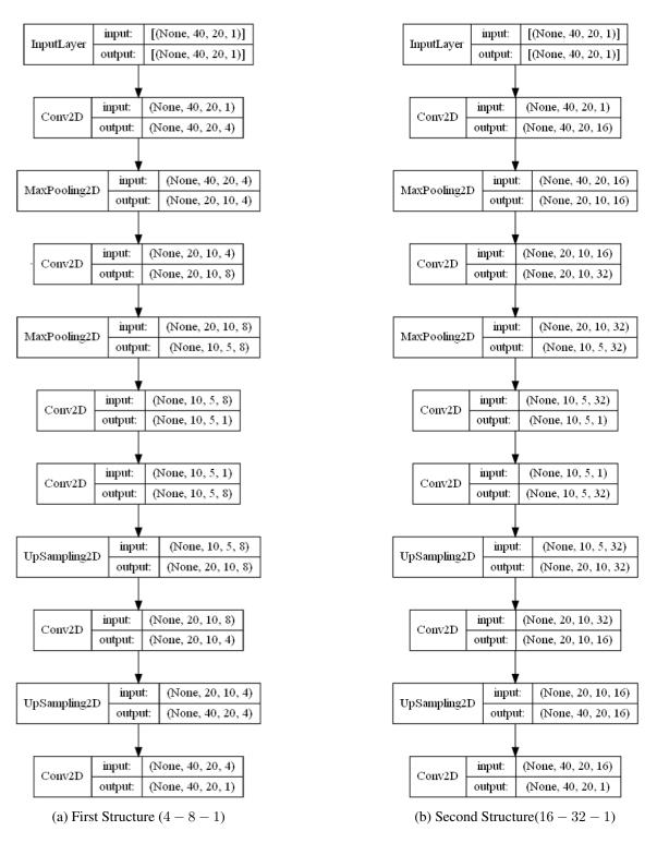
Figure 5.3: Convolutional Autoencoder configurations used in this study.
