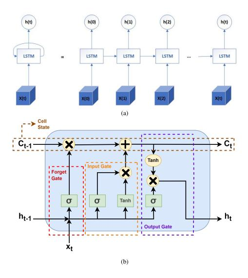
Figure 2.1: (a) Folded and unfolded LSTM network. (b) LSTM Cell
