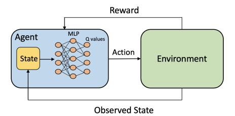
Figure 3.6: The block diagram of the DRL model.
