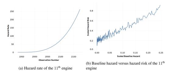
Figure 3.1: (a) Hazard rate corresponding to the  $11^{\text{th}}$  engine. (b) Baseline hazard (BH) versus Hazard Risk (HR) associated with the  $11^{\text{th}}$  engine.
