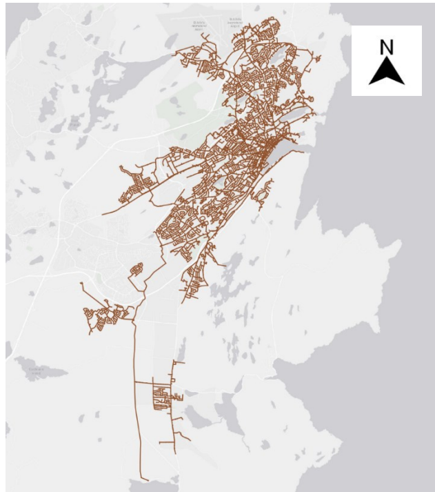
FIGURE 0.60 – ST. JOHN’S WATER DISTRIBUTION NETWORK (GIS FILE PROVIDED BY CITY OF ST. JOHN’S)
