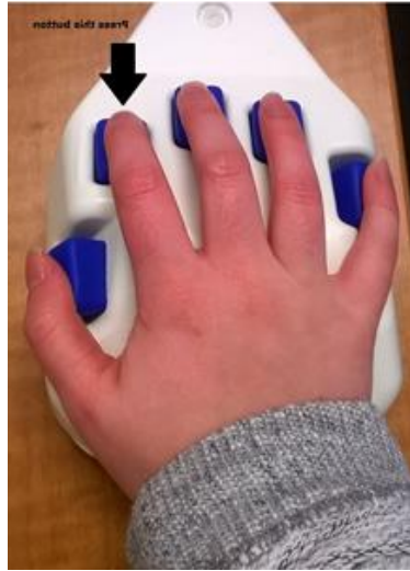
Figure 7: The response box used in the MRI scanner to interact with the tasks displayed on the mirror.
