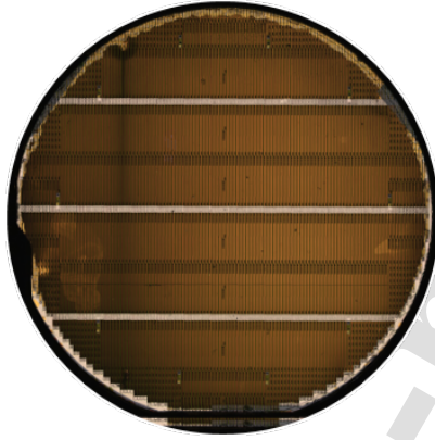
Figure 1: Optoelectronic wafer that contains multiple QCL devices.
