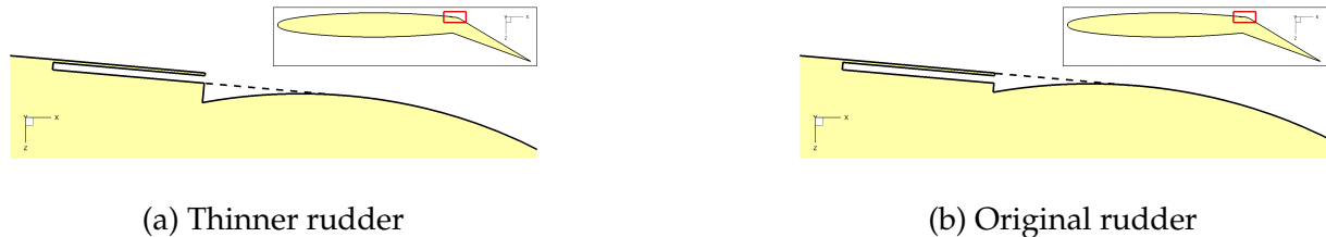
Fig. 4.8 Geometry in the vicinity of the slot with thinner and original rudder
