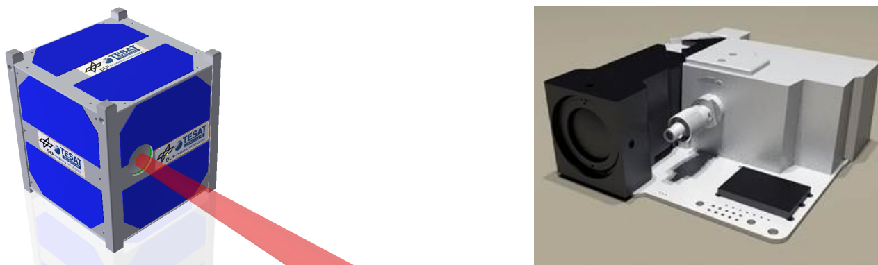
Figure 8: OSIRIS4CubeSat installed in a 1U CubeSat for illustration purposes (left); CAD model of the terminal (right)
