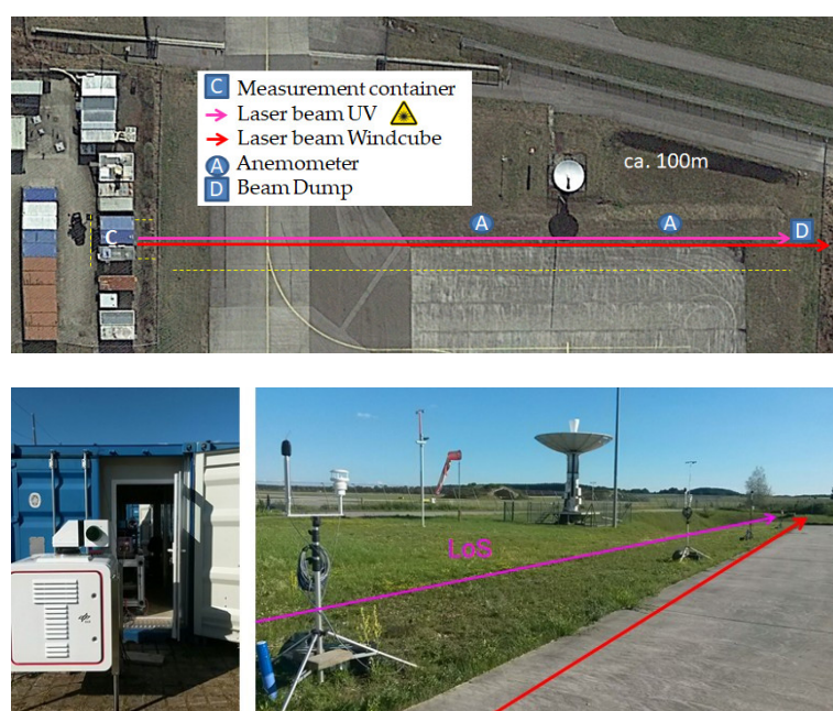
Figure 7. Setup of the ground test campaigns in 2017 and 2018.
