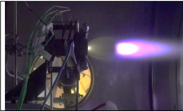
Figure 22: Thruster during firing in vacuum chamber
