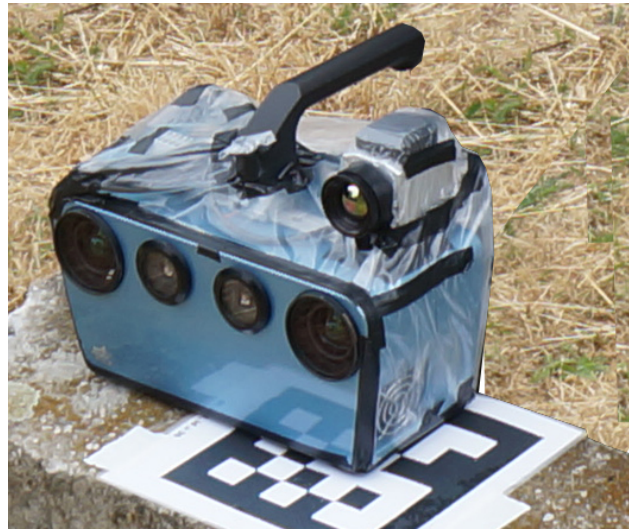
Figure 1. Trifocal IPS with a thermal (on top) and two visual cameras (front).
