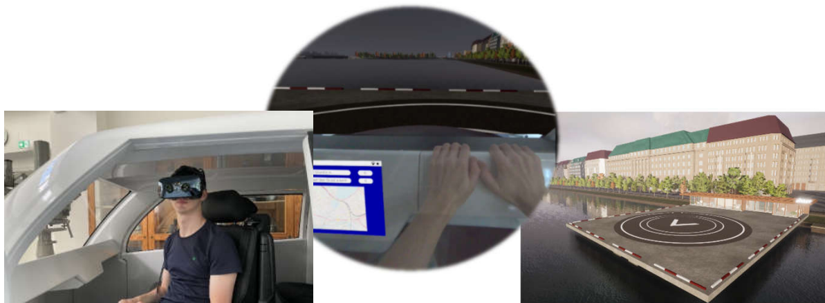
Simulator set-up with cabin mock-up and head-worn mixed reality display, virtual Hamburg scenery
