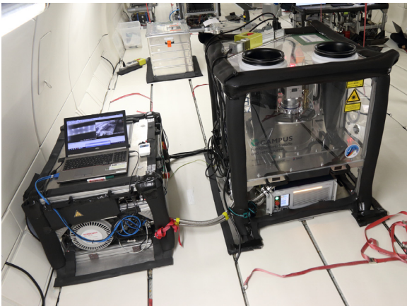
Fig. 4. Photo of the two racks setup for laser beam melting (LBM) at microgravity as mounted in the airplane (Rack 1 (right) includes the LBM system, rack 2 (left) vacuum includes the pump and computers to control the process).
