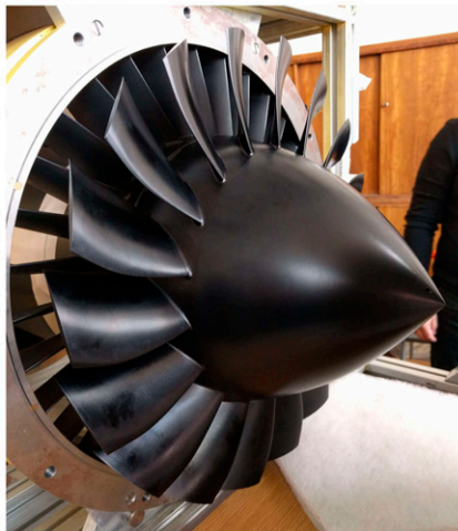
(c) Blade integrated disk rotor mounted on the Flocon test rig.
