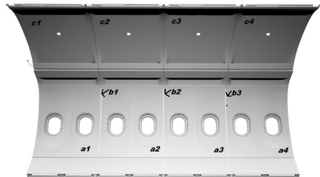
Figure 8 – Cabin lining components for assembly with different number of robots
