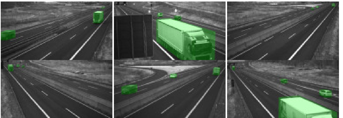
Fig. 6: Images of the on-ramp section near Cremlingen of the TFNDS with overlaid bounding boxes. The dataset used in this work is collected in that area for scenario extraction and analysis.
