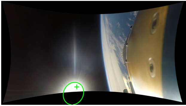
Fig. 28 Undistorted image of camera 2 on the ATEK sounding rocket at T+171 s with the ellipse that was fit to the selected undistorted Sun curve, and x- and y-coordinates of the estimated Sun direction vector \hat{\mathbf{e}}_c
