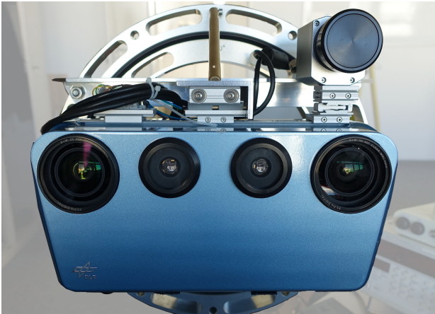
Figure 3. Stereo-Camera system with long-wave infrared camera attached on top. The system is mounted on a rotary plate for calibration purposes.
