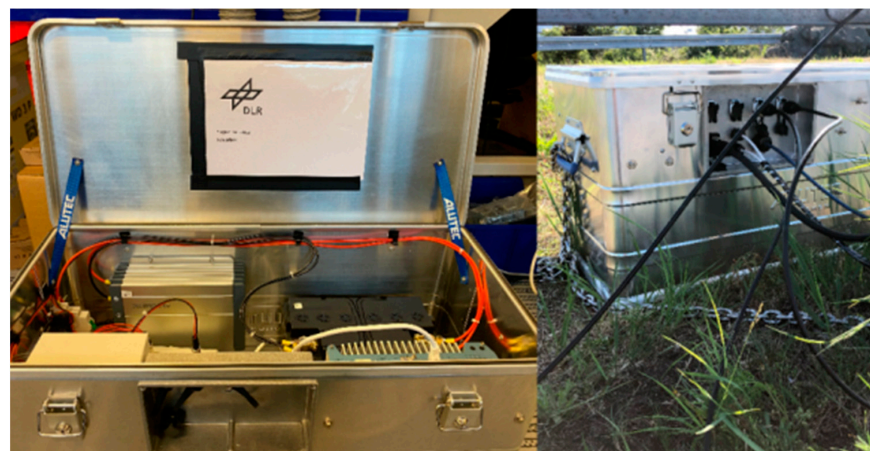
Figure 6. Sensor processing unit with battery backup that records the data from the LiDAR sensors together with various other sensors, such as AIS, camera, and weather-related information, and also communicates processed information via the mobile network.
