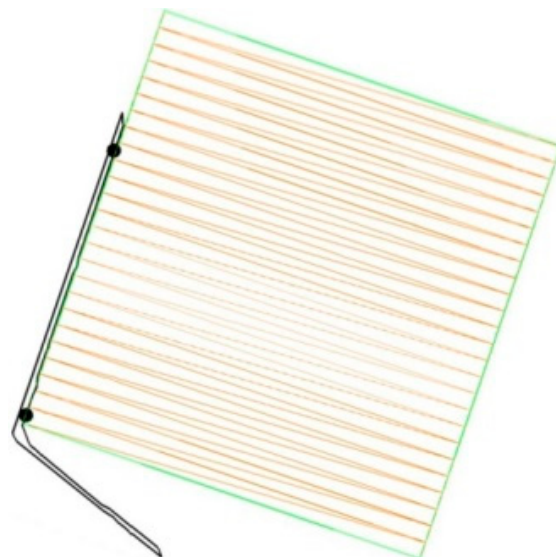
Figure 9. Quay wall model extracted from a point cloud. Black dots show the position of the LiDAR sensors. Polygon on the left shows the extracted quay wall shape. Orange boxes show the location and box filter of the defined vertical Reference Point filters. Additional horizontal Reference Point is marked as green rectangle.
