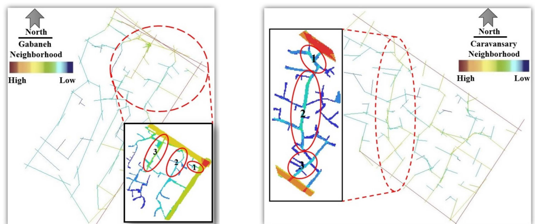
Figure 13. Identification of the most important streets that have to be reinforced in order to enhance the permeability within the neighborhoods and provide an influential interaction between 2D configurational attributes and 3D landmarks using incorporation of step 1 and step 3 of the research flow.
