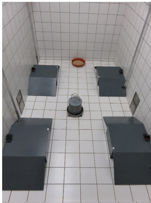
Figure 1. Test chamber with 4 traps (in this case without a safety station) on platforms covering the antenna logger system as well as a food tray and a drinking trough (during the conditioning period) and connected to the nesting chamber (not shown)
