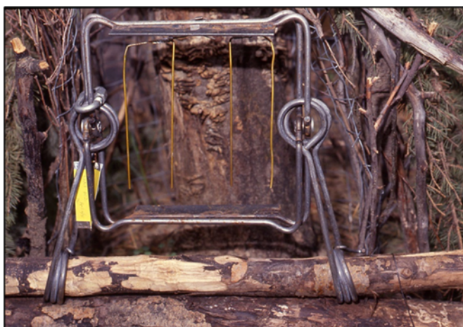
Figure 4. A modified Conibear 300 trap with pitchfork trigger for Canada lynx (Photograph: G. Proulx © ).
