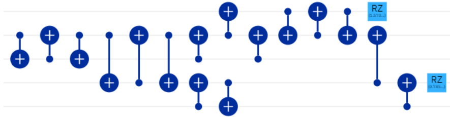
FIGURE 20. The representation of the transpiled quantum circuit for the quantum circuit in [26].
