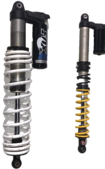
Figure 5.2 Prototype Semi-Active Damper (left) & Current Passive Damper (right)
