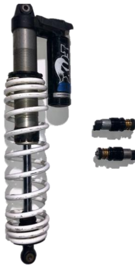
Figure 5.1 2.5" OD x 7/8" Shaft Fox Damper & Fox Live Valve Adjuster
