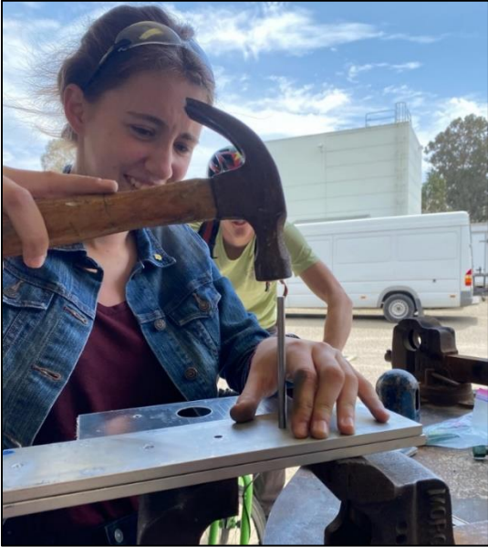
Figure 7. Peyton using the fin bending jig to flare a hole in a fin prior to soldering.
