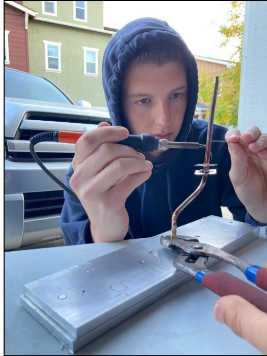
Figure 4. Kadin doing initial soldering test with a test token. All test tokens on the heat pipe were different shapes and sizes.
