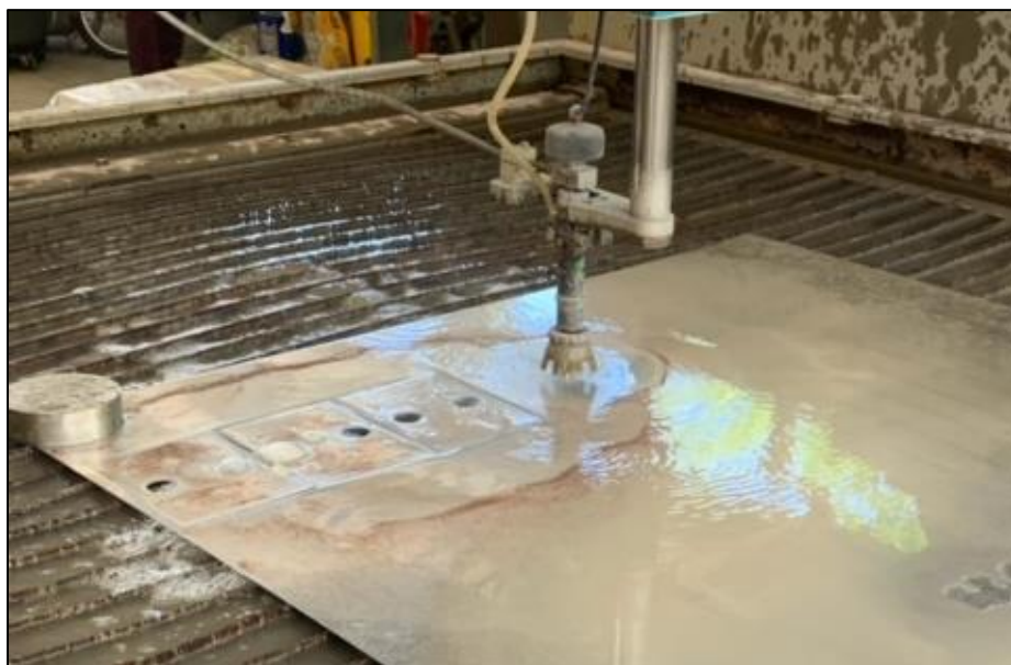
Figure 5. Water jet cutting heat fins from aluminum sheet.
