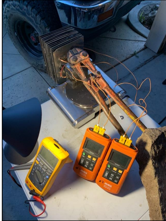
Figure 10. Test setup for nighttime ambient conditions. The bolt cutters and locally sourced diorite rock were critical to ensure test fixture stability.
