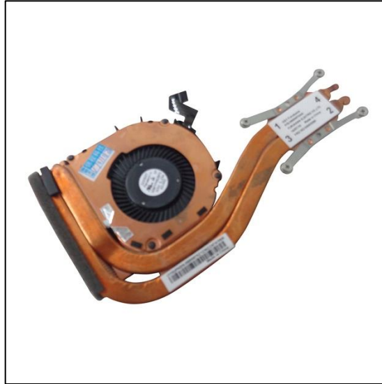
Figure 1. A Common Laptop Heatsink Solution. [1]
