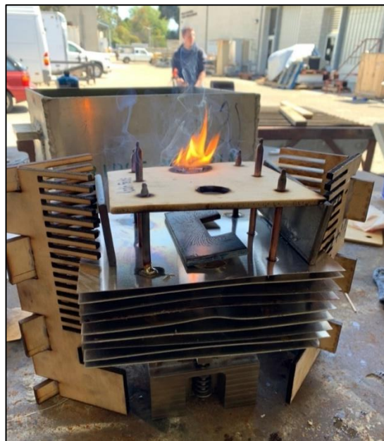
Figure 9. Limitations of wooden jigs.
