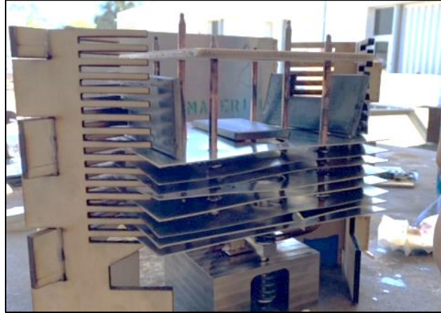
Figure 8. Heat fins are being soldered to heat pipes. Wooden jigs pictured on left and righthand sides.
